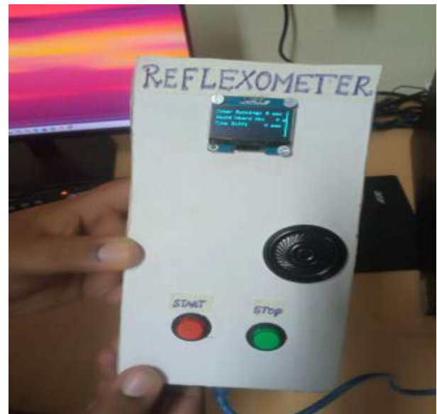
Fig. 4. Developed reflexometer hardware prototype.
