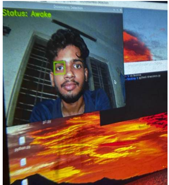
Fig. 3. Real time driver monitoring interface using Haar cascade
