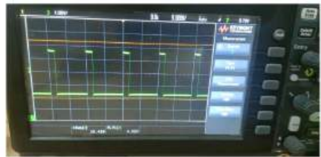
Fig. 5. PWM Output Waveform Captured
