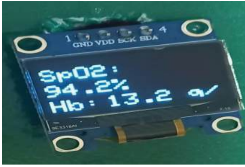
Fig. 4. OLED Display Showing Real-Time SpO 2 and Hemoglobin Output
